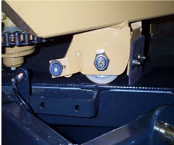
MAGNET AND ROTATE SENSOR ROTATE SENSOR –PART NO,ZLY-PO6. MAGNET-PART NO, D6043
