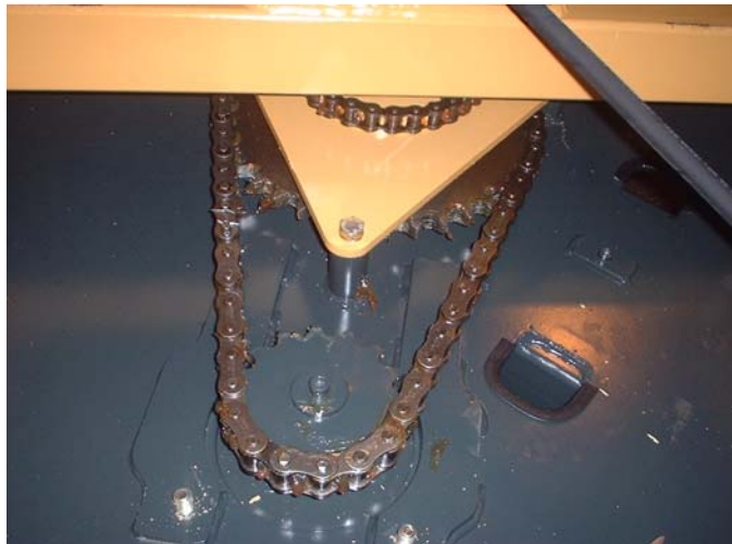
MAIN DRIVE CHAIN, CENTRE SPROCKET AND MOTOR SPROCKET.
